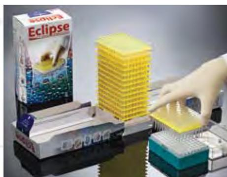
**2.** Align transfer top over refillable rack and place onto rack.
